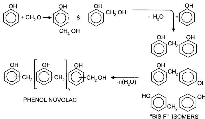
functionality of two. The epoxidation of phenol novolacs yields a mixture of di- and poly-functional resins as shown in figure 3.
